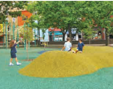
Phase 2 Rubber Surface Mounds and porous surface infiltrate stormwater
